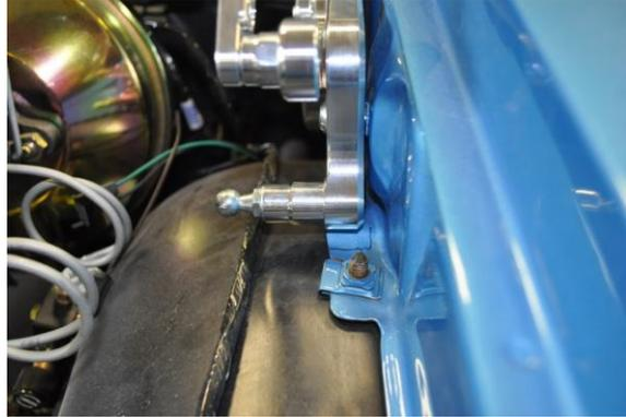
5. If the fender tab interferes with the hinge fender bracket it must be modified so that it will not interfere with the downward adjustment. A portion of the fender tab can be removed or flattened to gain the required clearance. To mark the portion that must be modified, loosely bolt the hinge on to the fender and trace around front portion of hinge.
